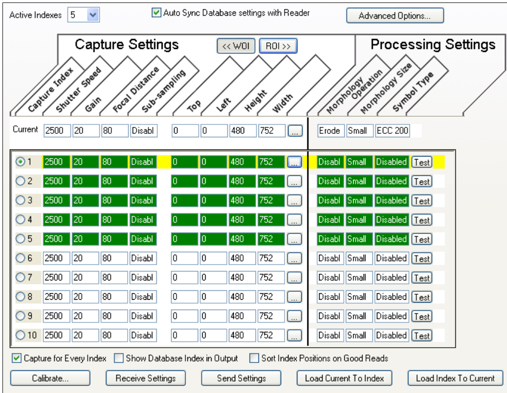
Configuration Database view, CMOS, set for 5 Active Indexes, with Capture Settings highlighted
