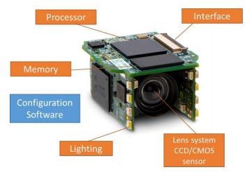
Figure 3: 2D Reader Components
