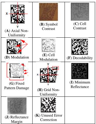
**Figure 2: Verification Evaluation Parameters**
