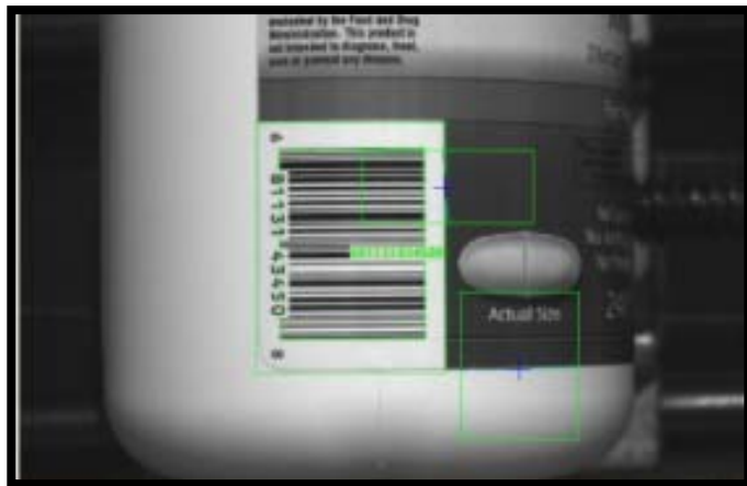
Read barcode and check label position
