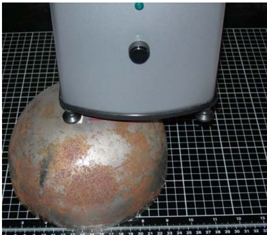
FIGURE C-4. Setting Up Correct Stand-Off Distance
