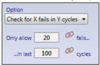
In the above example, the trend status output will turn on if there are ever 20 failures in the last 100 inspections.
