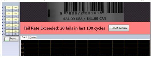
Click the **Reset Alarm** button to clear the banner, and to reset the trend counts on the camera. Output 2 will turn on when the alarm is triggered, pressing Reset Alarm will not clear Output 2 immediately, but it will clear on the next inspection cycle. The inspection will continue to run even if the trend alarm has been triggered.
