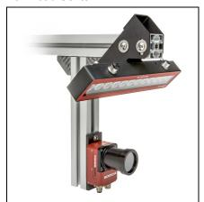
To achieve the most uniform lighting possible in an image, the light should be as far away from the region of interest as possible while maintaining a 45 degree angle and achieving adequate illumination.
