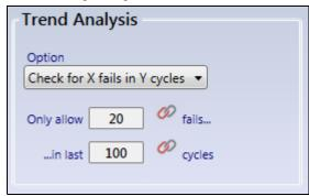
If the selected trend is detected, the job can be configured so that a digital output on the smart camera will turn **ON**. This can be configured by going to the **Tools** tab, selecting the **Inspection Outputs** tool, and looking at the **Digital Output** selections:
