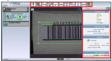
You can now insert tools into your job if necessary, and adjust all parameters. When the Tools tab is selected, you have the same capabilities as you do in the Edit view of standard AutoVISION.
