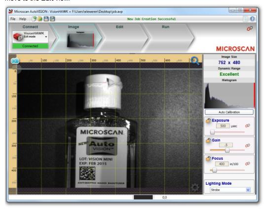
You can return to the **Connect** view and click the **Modify** button to adjust additional camera settings, such as **TCP/IP** settings, **RS-232** settings, **Ethernet** settings, **Industrial Protocol**, and **AutoVISION button** settings. You can also rename your camera (alphanumeric characters only - [0-9], [a-z], and [A-Z]). Click the **Apply** button when you have adjusted the camera's settings as needed.
