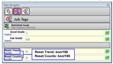
If the **Link** icon is clicked, the linked value can be changed to a value that can be addressed by a PLC using EtherNet/IP or PROFINET industrial protocols. Once the links to these items are changed from the defaults, the VMI user interface functionality associated with these items will be effectively disabled due to the Link value superseding the user interaction.
