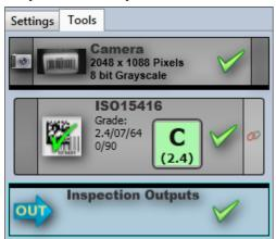
The **Inspection Outputs** tool is used to communicate the results of your inspection to the outside world. You can output results via **Digital I/O**, or as string data sent via the **serial port** or the **Ethernet port** (via **TCP/IP**).
