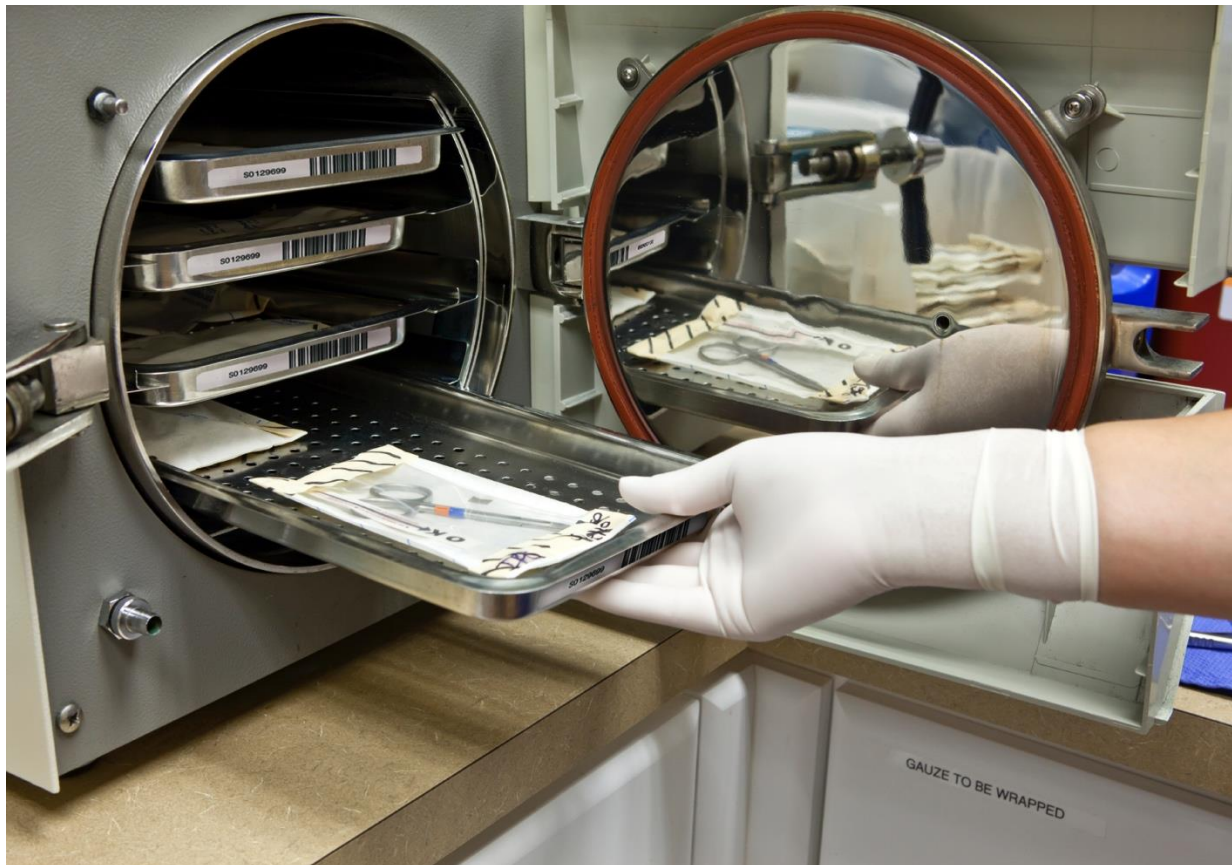
Figure 3: A hospital worker places a set of surgical instruments into an autoclave for sterilization. Each of these instruments will soon need to bear DPMs that can withstand multiple sterilization treatments.
