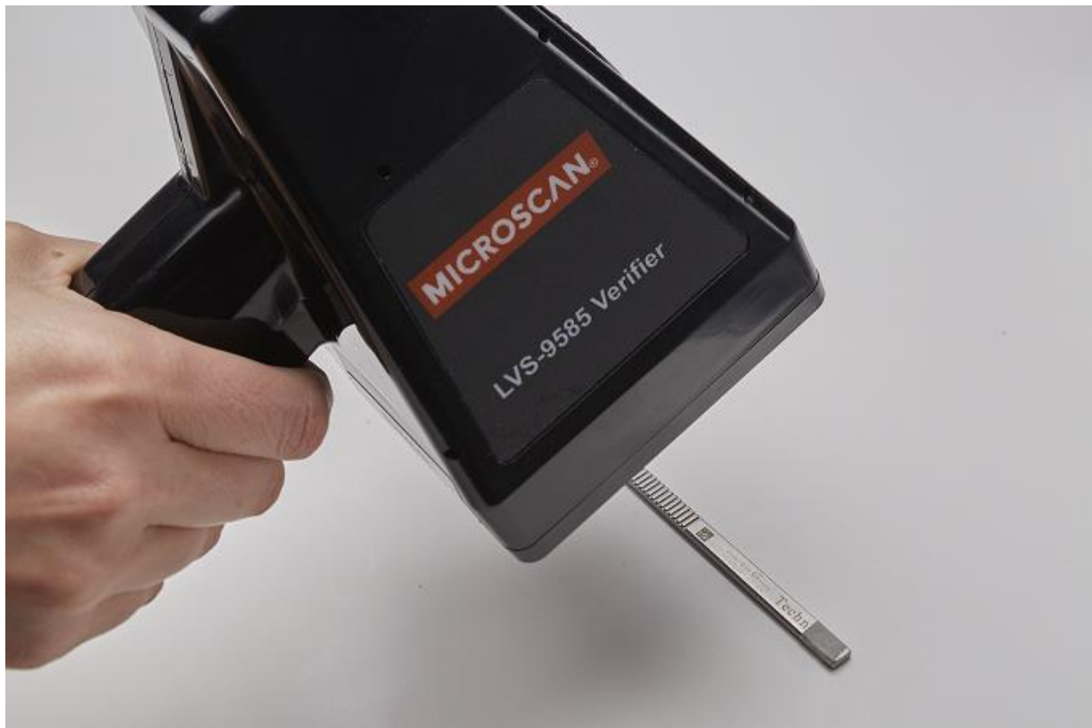
Figure 7: A handheld verifier checks the readability of a minuscule DPM.
