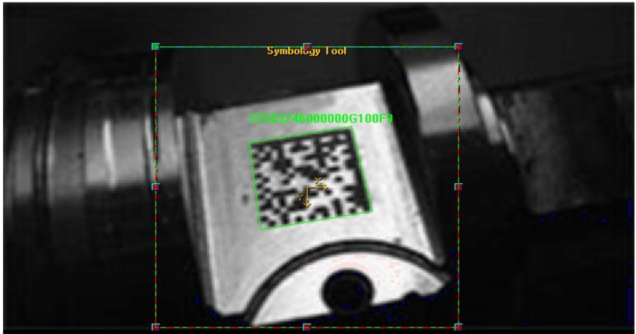
Figure 6: A Data Matrix on a metal surface. Can you spot the finder pattern and the timing pattern?
