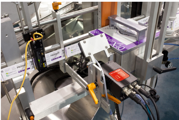
Figure 14: Verification steps can be added at any point along the line to guarantee label quality wherever errors may result and the verification system may contribute to cost savings.
