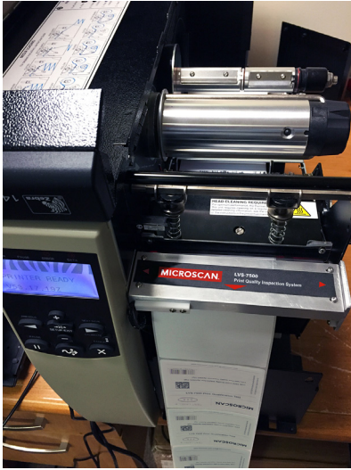
Figure 13: An inline verification system is attached directly to a Zebra® printer to ensure label accuracy while printing.
