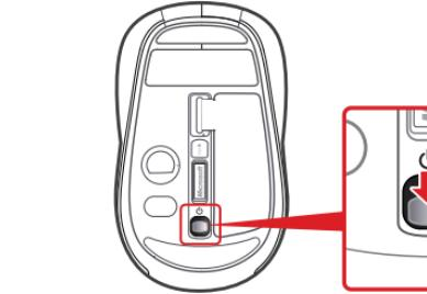
When not in use, turn the mouse off to extend battery life.
