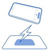
Qi works using magnetic induction, and is currently designed for devices that use 5 watts of power or less, such as mobile phones. Qi chargers and devices use the same frequency, so as long as their active areas are touching, all Qi products are compatible, regardless of manufacturer or brand. For more details, see the user guides of both devices.
