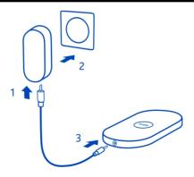
Use the charging plate only with the supplied power supply.
