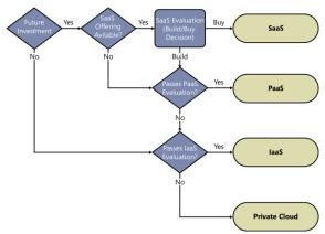
Figure 4-4: High-level workload placement decision tree
