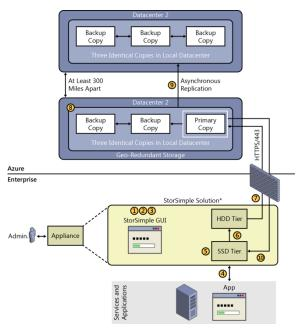
Azure StorSimple is a storage solution that uses both an on-premises appliance and Azure. As shown in the illustration:
