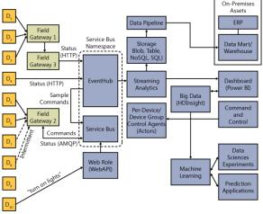
Figure 5-6: A rich end-to-end IoT application
