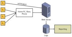
Figure 5-5: Simple IoT architecture
