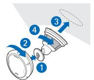
If the ambient temperature is below  $+15^{\circ}C$  (60°F), carefully warm the surface and the suction cup with a hair dryer to ensure a firm grip on the windscreen. Ensure that you do not heat the windscreen excessively to avoid damage to it.
