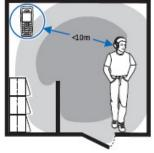
picture. The connection is subject to interference from distance and obstructions (shown in light grey) or other electronic devices.
