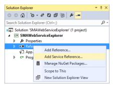
5. In the Add Service Reference dialog box, type the URL of the web service, for example type https://sma.contoso.com:9090/0000000-0000-0000-0000-0000000000, and then provide a name for the namespace, for example type SMAWebService.
