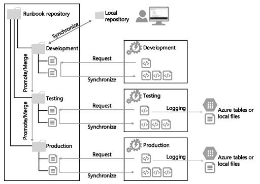
FIGURE 6-7 Continuous integration model
