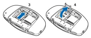
**5** Insert the SIM card into the SIM card holder (5).
