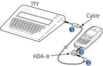
3 Plug the HDA-8 into the connector on the bottom of your phone
