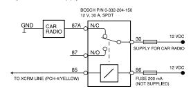
Another possibility is to use a special muting unit, which mutes the radio by connecting load resistors (not included) to the speaker lines of the car radio.
