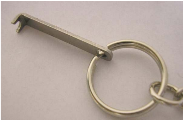
Figure 7: Antenna Extraction Jig
