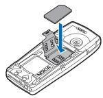
Close the SIM card holder and press it until it snaps into position.
