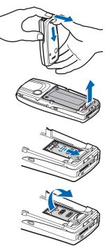
6 Insert the SIM card into the SIM card holder with the beveled corner to the top left and the gold contact area facing down.
