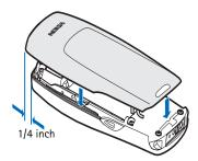
4 Press down slightly and slide the cover until it locks into place.
