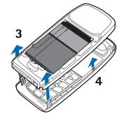
5 Gently push the cover latch on the top of the front cover through the locking hole in the top of the phone and snap the cover into place.
