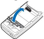
3 Insert the SIM card into the holder as shown, beveled corner first, with the gold colored contacts on the SIM card face up (away from the phone).
