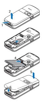
To remove the battery, lift the lower end of the battery out of the compartment (7).
