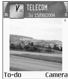
Fig. 1 Standby mode with a new background image, a new selection key shortcut, and Bluetooth activated.
