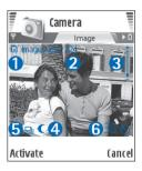
In the Sequence mode indicator (5) shows that the camera is in sequence mode.
