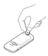
To release and replace the back cover, turn the screw with a coin or screwdriver.
