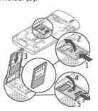
Ensure that the contact area on the card is facing down on the device, and the bevelled corner is facing down in the SIM card holder.
