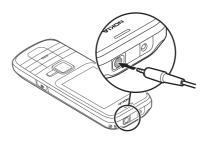
**Connect a USB data cable**Connect a compatible USB data cable to the USB connector.
