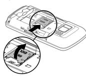
4 Insert the SIM card into the card holder. Make sure the contact area of the card is facing down.
