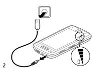
To avoid breaking the charger connector, be careful when connecting or disconnecting the charger cable.
