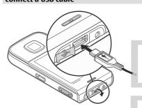
Open the cover of the USB connector, and connect the USB cable to the device.
