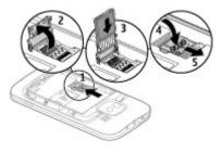
3 Insert the memory card, with the contact area facing down.
