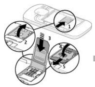
4 Line up the battery contacts, and insert the battery.
