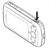
To capture an image, press the capture key. Do not move 3 the device before the image is saved and the final image appears on the screen.
