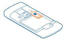
Line up the battery contacts, and insert the battery.
