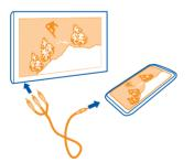
Do not connect products that create an output signal, as this may damage the device. Do not connect any voltage source to the Nokia AV connector. If you connect an external device or headset, other than those approved by Nokia for use with this
