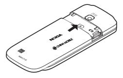
**Important:** To prevent damage to the SIM card, always remove the battery before you insert or remove the card.
