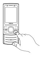
Press and hold the power key to switch the device on and off. Press the power key briefly to end a call or close an application.
