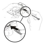
If the SIM card is not properly in place, the device can only be used in the offline profile.
