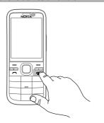
Press and hold the power key to switch the device on and off. Press the power key briefly to end a call or close an application.
