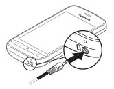
3 When the device indicates a full charge, disconnect the charger from the device, then from the wall outlet.
