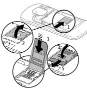
Line up the battery contacts, and insert the battery.
