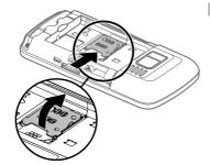
4 Insert the SIM card into the card holder. Make sure the contact area of the card is facing down.
