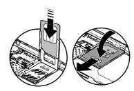
6 Line up the battery contacts, and insert the battery.
