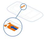
6 Line up the battery contacts, and insert the battery.
