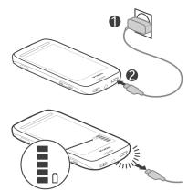
Tip: If there is no wall outlet available, you can also charge over USB. Use a compatible USB data cable to connect your phone to a compatible device, such as a computer. You can also copy data while charging.
