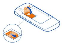
4 Line up the contacts of the battery and the battery compartment, and insert the battery. To replace the back cover, direct the bottom locking catches toward their slots (1), and press the cover, until it locks into place (2).
