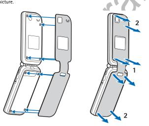
To remove the wrap, first loosen it from both sides of the hinge (1), then from the ends of the phone (2).
