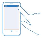
Silent mode (a) is switched on. If you have set your phone to vibrate, vibrate mode (b) is switched on instead of silent mode.
