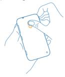
2. Slide the memory card holder until it unlocks, and lift the holder.
