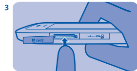
3 Push the card in until it locks into place. Close the cover.
