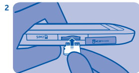
2 Put the memory card in with the contact area face up.
