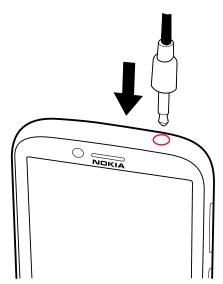
Do not connect products that create an output signal, as this may damage the device. Do not connect any voltage source to the audio con-
