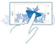
To focus on a specific object or area, tap the object or area on the screen. Hold the phone still until the white square stops blinking.
