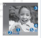
• Image stabilizer (4) indicates that the image stabilizer is active, and dampens the effects of small movements on the image sharpness (main camera only).
